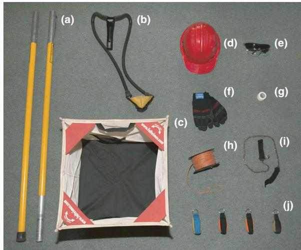
**Fig. 1.** Basic equipment: A Big Shot throw-line launcher (SherrillTree Inc.), which is comprised of two, four-foot connectable Jameson fibreglass poles (Jameson Inc., (a)) and a rubber head with pouch (b), line storage bag (c), hard hat (d), safety glasses (e), gloves (f), medical tape for wrapping fingers (g), lightweight but sturdy nylon line (h), flexible saw (i) and weighted bags between 8 and 16 ounces (j).
